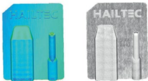
3D measurement of an embossing stamp with AI-supported measurement technology: The CAD deviation can be displayed with false colors or target-actual comparison.
